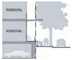
FIGURE 14: Maximum height that ground floor may be raised above finished footpath level UDG V3.0
