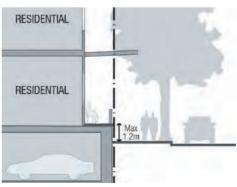
FIGURE 46: Maximum height of semi-basements above finished street level
