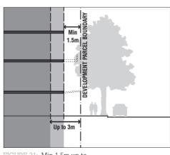
FIGURE 21: Min 1.5m up to Max 3m Street Setback Section
