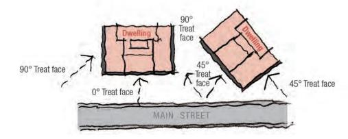
FIGURE 50: Determination of treated facades
